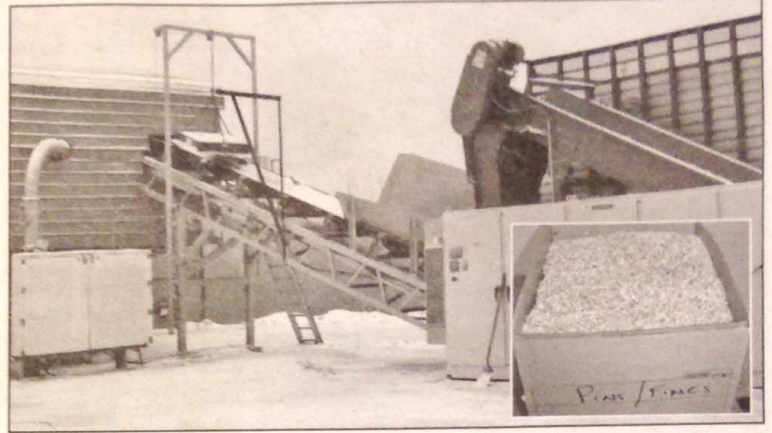
After the wood is chipped, the pieces are pushed onto the conveyor, where a magnet pulls metal from the chips. The chips are then put through sifters that take out the pins and fines (inset) or other unwanted items. Chippewa River Forest Management (CRFM) built a wood chipper plant in Cornell to cut cost to the primary mill. Mule-Hide Products, Cornell, and CRFM work together to update and improve their companies. (Photo by Kayla Peche)
