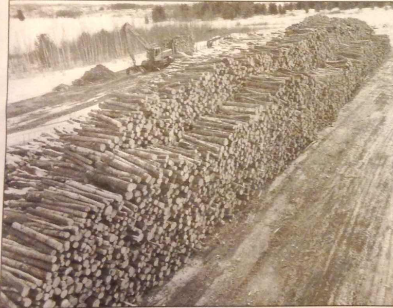
During the winter months, Chippewa River Forest Management collects a large number of roundwood, which is used during the slow harvesting months. The loader takes the logs to the chipper to be cut and screened, then hauled to the mill. (Submitted Photo)
